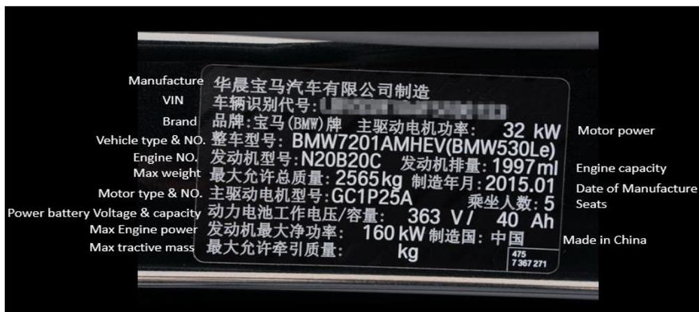
The label must meet the requirement GB/T25978 and GB-16735. There are 3 VIN identifiers on a vehicle. First is on the label, the second is on the windshield, and the third is on the front panel. In addition, the vehicle certificate will have VIN and engine number.
