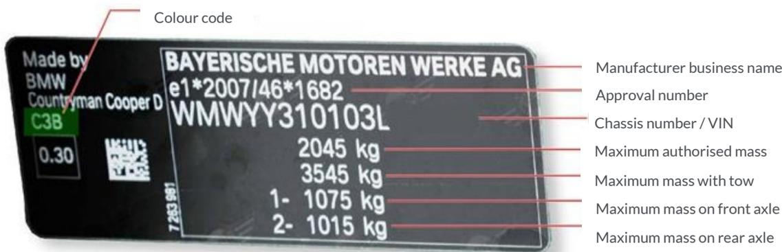
The manufacturer label is shown to be attached to the base of the right (driver-side) centre pillar. There are additional VINs located on the left side of the vehicle under the windscreen and die-cut in the turret on the suspension. The tyre pressure label is attached to the left (passenger-side) centre pillar.
